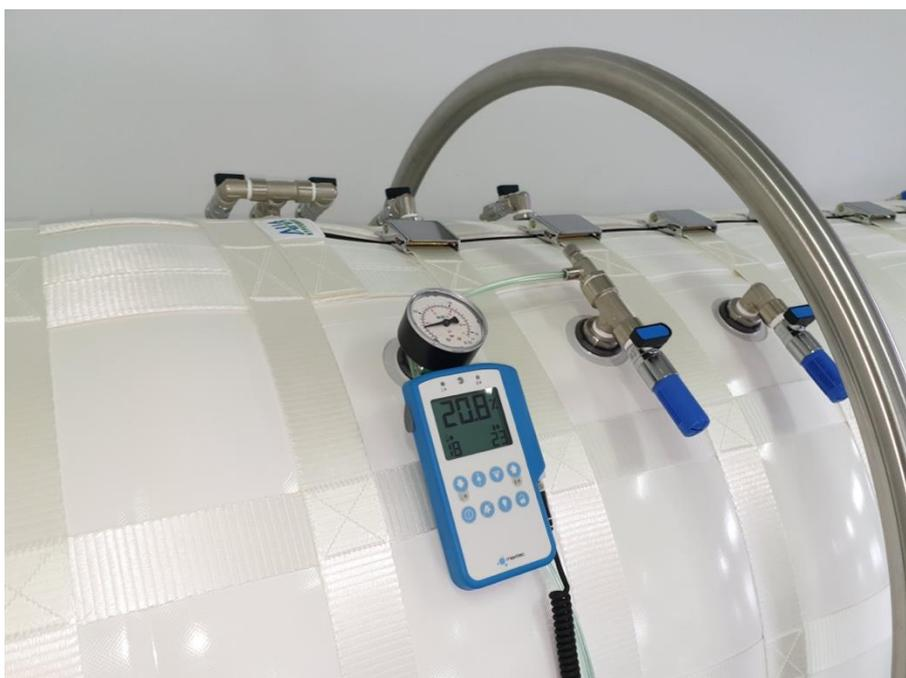
*Oxygen monitoring analyser with alarm*
